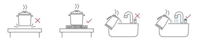
**Boiling liquids:** If you pour boiling liquids into HI-MACS® sinks or basins, you should also pour in cold water at the same time.
